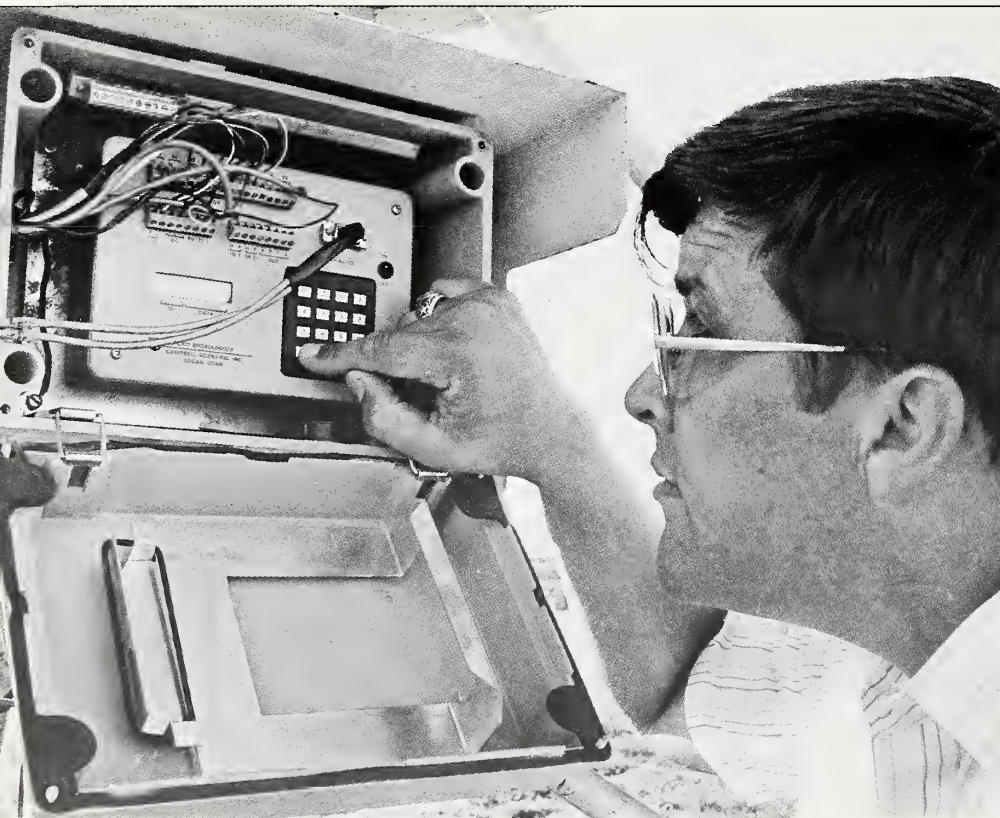
Above: Terry Howell, agricultural engineer, programs a weather station computer for solar radiation, wind, air temperature, and humidity readout. This system monitors measurements from weather data instruments and delivers them to the main computer. The main computer then processes this information in order to deliver the right amount of water to the field (0781X879-8).
