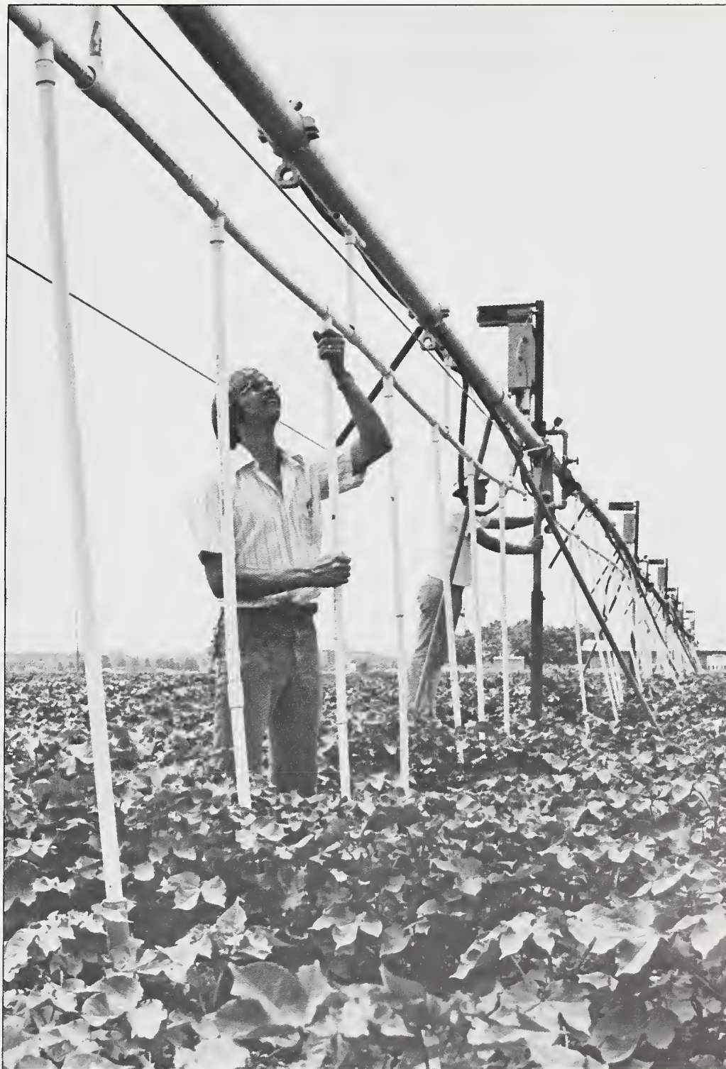
Top left. Automating the irrigation system almost completely, this main tower computer system controls water allocation, reads water meters, and turns system on and off. Heimann, assisted by Sikorski, checks one of the system's programs (0781X878-23).
